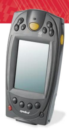
The PPT 2740 integrates Spectrum24®, Symbol's IEEE 802.11-based wireless LAN technology for real-time data communications with your remote host system.
